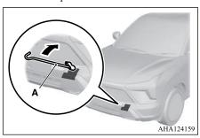
3. Use the jack bar to firmly attach the towing hook (B).
