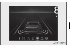
The ON/OFF status of each driver assistance system is displayed. Press the Left switch or Right switch, select the function setting display of the multi information screen. Each system can be turned ON/OFF on the Driver assistance menu screen.
