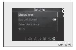
"Display type", "Sub unit speedometer", "Driver assistance", "TPMS", "Pop-up notification", "Ambient lighting", "Tailgate", "Rest reminder", "Turn-signal sound", etc. can be changed to the setting of your choice. Please follow the procedure below.
