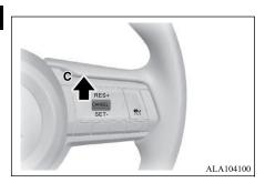
To increase your speed in small amounts, push up the "RES +" switch (C) for less than approximately 1 second and release it. Each time you push up the "RES +" switch (C), your vehicle will go 1.0 km/h faster.
