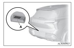
• When the operation mode of the power switch is ON, the electric tailgate cannot be opened by pressing the open switch, unless the select position is in the "P" (PARK) position.
